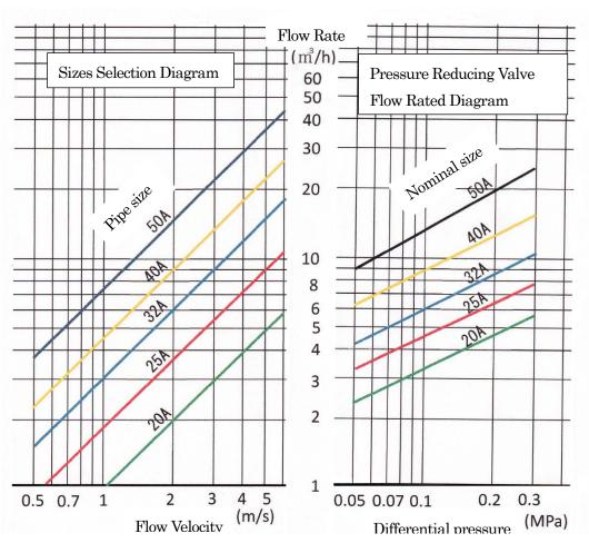
(Note) To consider the noise occur and durability, the ideal piping flow velocity is under 2m/s
