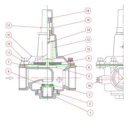
With adjustment of the outlet pressure, 7 diaphragm and valve assembly (5 seal, 3 plunger) will keep the balance, self adjust the valve opening to maintain the outlet setting pressure.
