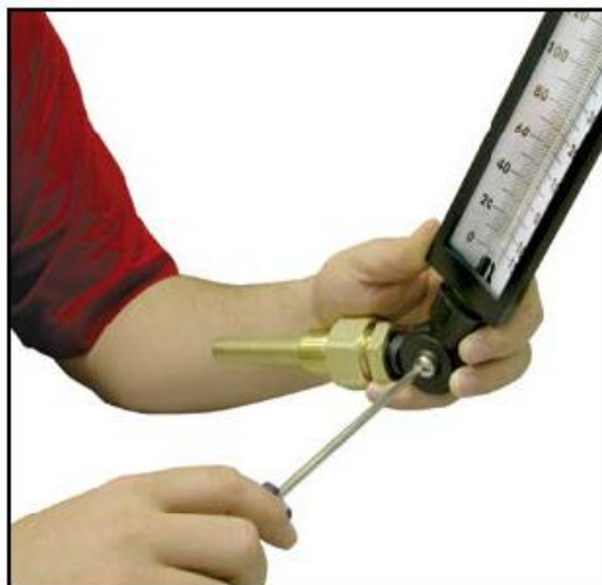
Tighten screw (A) to secure the angle.
